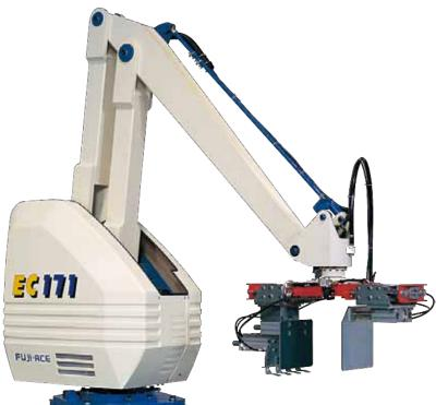
The most popular in the FUJI-ACE line, the **EC-171** robot has the largest working envelope, while maintaining the smallest rotation radius. Energy-efficient, as it uses only 4KVA, able to operate in tight spaces while still accomplishing high palletizing rates, it is ideal in most palletizing applications.
